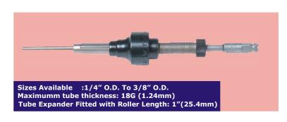
For Tube Inside Diameter From (3.8mm) .152" to (8.4mm) .331"
